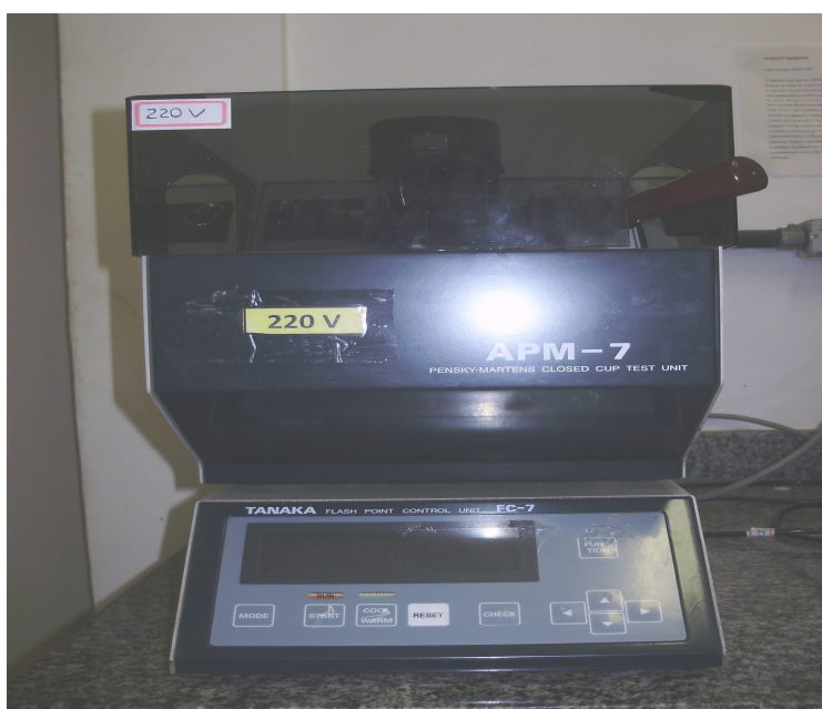
Figura 4.3. Medidor de ponto de fulgor Pensky Martens closed Cup Test Unit
